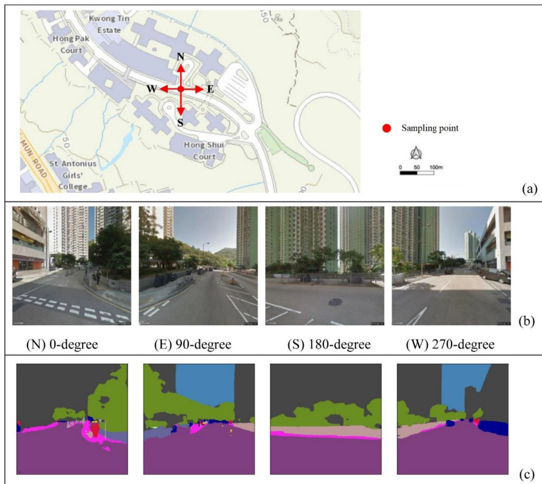
Fig. 2. Eye-level street greenness assessment with PSPNet, a computer deep learning technique. (a) Sampling points with 50 m spacing were generated in the street centerlines. (b) Four streetscape images were retrieved for each point from Google Street View, in the north, east, south, and west directions, respectively. (c) All street vegetation in the images was segmented with PSPNet.
