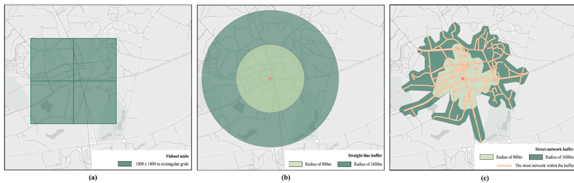
Fig. 1. Three methods for greenspace exposure measuring. (a) Measured with fishnet units (or district, zip code); (b) Measured with straight-line buffer; (c) Measured with street-network buffer. Aggregate measure (a) (e.g., fishnet units, district, zip code) is typically used in collective greenspace-mortality studies but may be affected by ecological fallacy and lead to inconsistencies and misinformation. Straight-line buffer (b) is typically used in individual greenspace-mortality studies, assuming that individuals can walk around freely within the buffer. Street-network buffer (c) considers the street network with a more detailed representation of the area around the individual.
